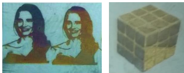
Figure 2. An example of the colour image obtained by laser oxidation on a surface of polycarbonate film coated with a thin layer of titanium.
