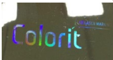
Figure 1. Photography of the picture formed on the Ni film by laser exposure
